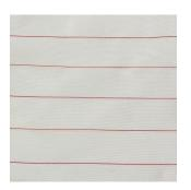
Airtech's Econostitch® is an economical, heat set and scoured peel ply with good performance when used with both polyester and epoxy resins. It features red tracers for high visibility before and after cure, reducing the possibility of the peel ply being left of the part.
